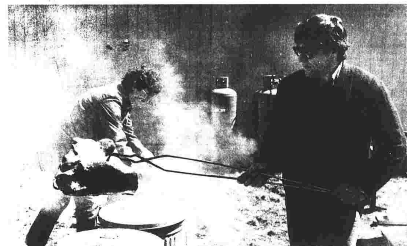
Stevens holds a red-hot piece of pottery with tongs just after he took it from the student-built kiln. The melted glaze is ready to be textured in one of the pails.
